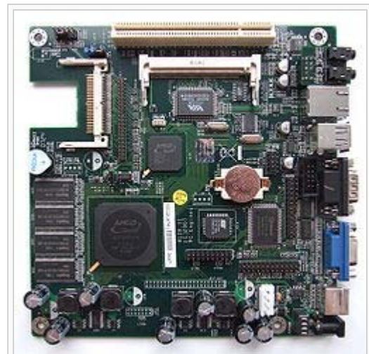
PC Engines' ALIX.1C Mini-ITX embedded board with AMD Geode LX 800 together with Compact Flash, miniPCI and PCI slots, 44-pin IDE interface and 256MB RAM
