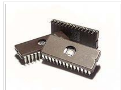
Microchips (EPROM memory) with a transparent window, showing the integrated circuit inside. Note the fine silver-colored wires that connect the integrated circuit to the pins of the package. The window allows the memory contents of the chip to be erased, by exposure to strong ultraviolet light in an eraser device.
