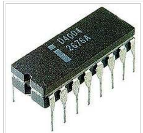
Intel 4004, the first general-purpose, commercial microprocessor
