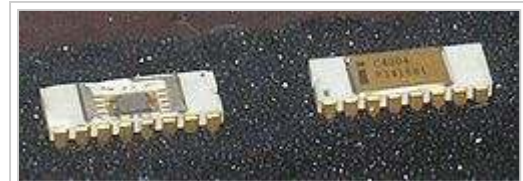
The 4004 with cover removed (left) and as actually used (right)
